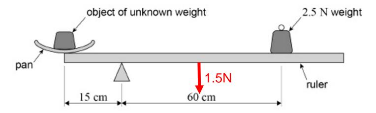
A scale pan of weight 0.5 N is placed at the end of the ruler and an object of unknown weight is placed in the pan. The ruler moves to a steady horizontal position when a weight of 2.5 N is added at a distance of 60 cm from the pivot as shown.
