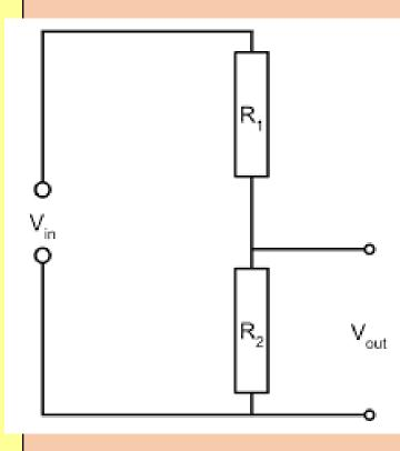
$$V_{in}/(R_1 + R_2) = V_{out}/R_2$$
