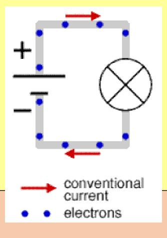
Electrical energy is used to do work in the circuit (e.g. transferred to light and heat energy)
